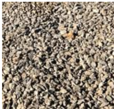
Image 12: Rock that is 20 – 40mm in size and free from dust and fines is used to backfill trenches
